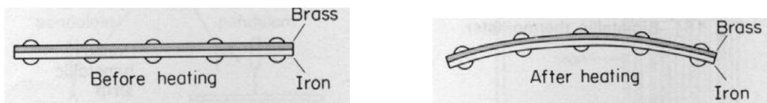
There are many problems faced by this phenomenon of expansion of solids. Bridges are built with a few inches of 'breathing space' at each end to allow the concrete and metals to expand in hot weather. This avoids cracking. Railway lines used to be laid with spaces at each end for expansion. Today they are made to join, with expansion spaces further apart. One positive use of expansion in metals is in thermostats.
