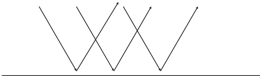
With a diffuse reflection the surface of the reflecting material is such that it has tiny irregularities on its surface so that when the ray hits the surface it is not properly reflected. In some cases the rays are very diffused indeed. Try an experiment where you shine light on different surfaces. See how some surfaces reflect quite well whilst others, like paper, do not reflect but diffuse the light.
