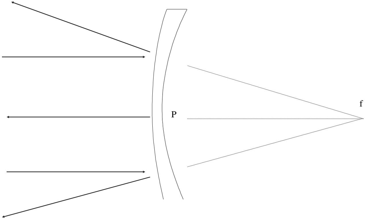
With a convex mirror the focus is **virtual**. This means that it is behind the mirror and is not real in the same way as a focus in front of a mirror is. The rays hit the convex mirror and are reflected off wider. The effect of this is to magnify the image.
