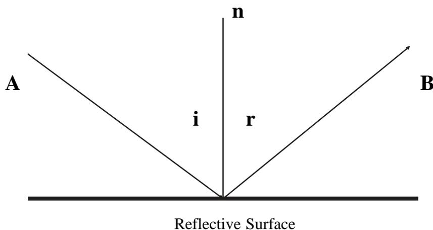
In the example shown above, the incident ray is the one marked 'A', and the reflected ray is the one marked 'B'. Sometimes you may be asked what the **angle of incidence** is or the **angle of reflection**. These are the angles which are formed between the normal, expressed as 'n', and the surface. Angles of the rays of incidence and reflection are marked above by 'i' and 'r'.
