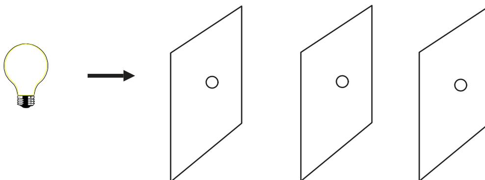
Shining a light, place pieces of cardboard with a small hole cut out, at intervals. Make sure that the small holes in the cardboard pieces are in the same place and lined up. Thread a piece of string through the holes to line them up. When you look through the holes you can see the light. If you move the cardboard pieces out of line, the light will be blocked and will not show.
